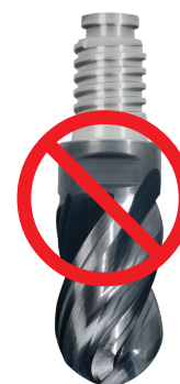
When surface profiling with any ball nose end mill, optimum performance will be achieved by tilting away from the center of the tool if possible.
